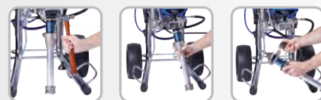
Loosen the Clamping Nut Open Door & Remove Pump Remove Hose & Suction Tube
